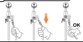
Move the device along the rope and check that it stays in position, then with one hand holding the lanyard or cows-tail, pull down vigorously to verify that the device locks on to the rope.
