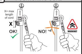
A positioning cord is factory fitted. If this becomes damaged or worn it can be replaced using cord. If 4mm cord is used it must be no longer than 40mm, 3mm cord must be no longer than 50mm. The only knot used must be to secure it tightly to the attachment point.
