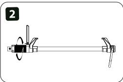
2. Fully loosen nut by turning counterclockwise.
