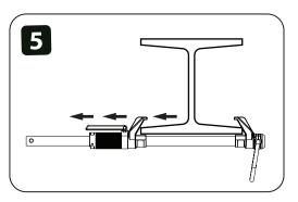
5. Pull back on adjustable paw to ensure it is in a locked position.
