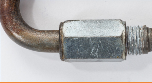
Quicklink with signs of oxidation and screw-up sleeve which you can't easily screw up.
