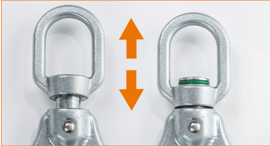
Connector has been loaded to more than 3 kN: the swivel can move far enough to cover the fall indicator. Service the anti-fall system containing the connector.
