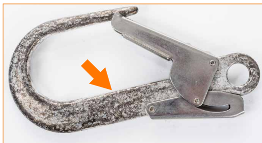
Double-lever connector with clear signs of corrosion.
