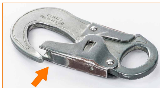
Oxidation on connector prevents closing catches functioning correctly.
