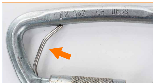
Connector with deformed ACL bar.
