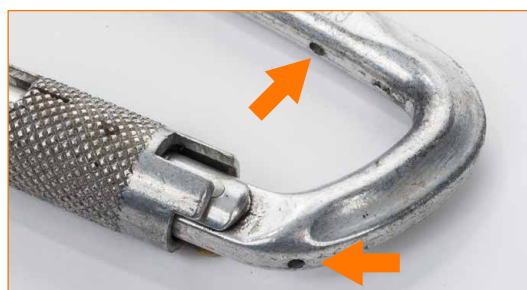
Connector with missing bar.
