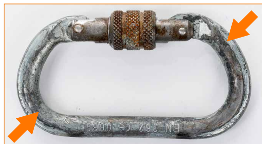
Connector with clear incision/cut on body.
