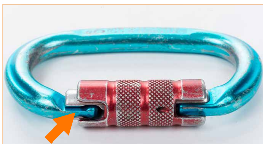
Connector with sleeve which doesn't automatically return to the locked position. 🛠️ Lubricate the sleeve as indicated in the user instructions. If the problem is not completely resolved, scrap the device.
