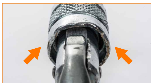
Connector with heavily damaged screw gate.
