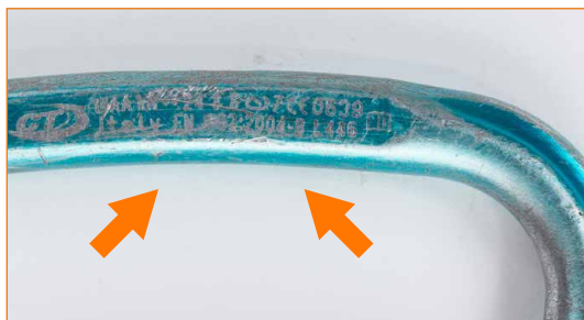
Connector's markings not completely legible.
