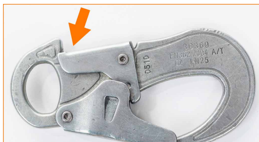
Double-lever connector whose rear safety lever doesn't return automatically into position.
