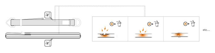
· Check the condition of the safety stitching on both sides. Look for any threads that are loose, worn, or cut.
