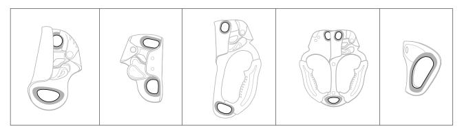
• Check for wear caused by rope running through the device.
