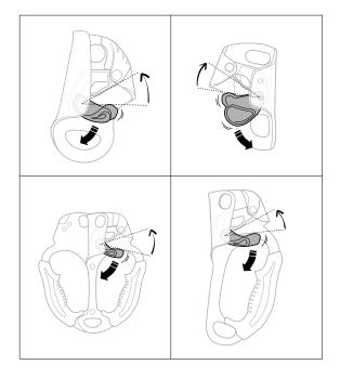
• Verify that the safety catch is able to hold the cam open.
