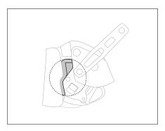
• Check the rotation of the wheel. Turn the wheel one complete revolution in both directions, making sure it rotates smoothly, without catching.
