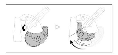
• Check the condition of the safety catches (marks, deformation, cracks...).
