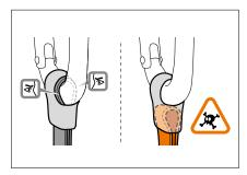
• Verify that the connector/sling/STRING assembly is correct.
