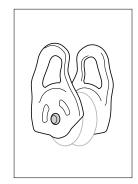
• Check the condition of the rivets (marks, deformation, cracks, corrosion, absence of play...).
