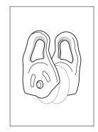
• Check the condition of the attachment holes (marks, deformation, cracks, corrosion...).
