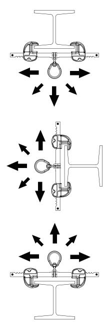
Placement at or below a user's working height requires integration of a compatible ANSI 359.1 shock-absorbing lanyard that does not allow the user to extend more than 6 feet (in any direction) from the anchorage connector before the shock absorber is activated. The beam anchor must be attached to the I-beam flange facing the user (top flange if above, bottom flange if below, etc.).
