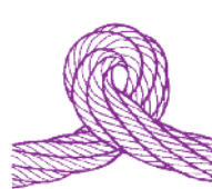
Kinked wire ropes which have been used. Kinks are pulled tight and caused distortion and failure.
