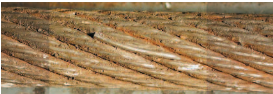
A single valley wire break on a 19x7 rotation resistant rope.
