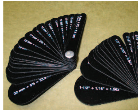
Correctly + 5% sized plastic and stainless steel sheave gauges available from Unirote.
