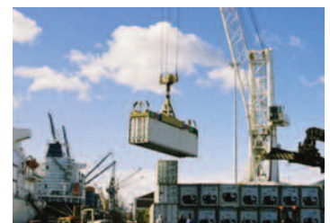
Python® Hoist non-rotating with plastic coated core to extend fatigue life due to shielding of core and strands. Plastic locks in factory applied lubricant.
