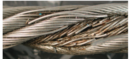
Example: Valley wire breaks on a 8-strand overhead crane wire rope
