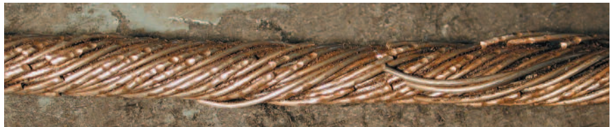
Condition of core under that same single valley break. Note the extreme notching of individual wire and the countless wire breaks. Such a condition is hidden under just a single (1) valley break !
