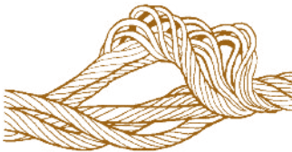
Bird Cage forced through a tight sheave.
